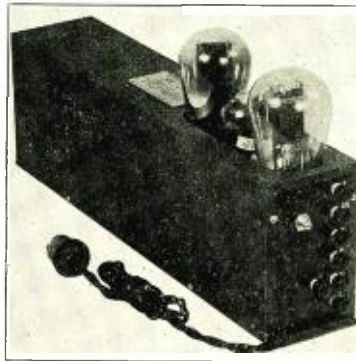
Fig. 1. A compact socket-powered amplifier with one '26, one '50, and one '81 tube.
